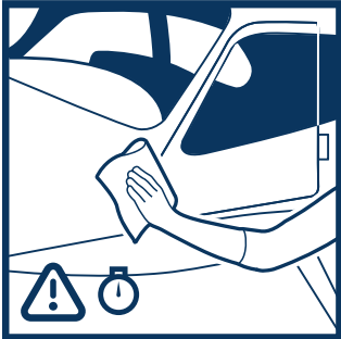
Wipe off immediately (10 ~ 30 seconds) after applying to the whole panel/section. Inspect each panel for high spots immediately.
