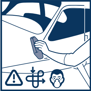
Apply a thick layer of Q² AERO. Level the coating well. Apply in your preferred motion. Levelling is crucial, not the application pattern. We recommend applying full panels. Split panels only while applying at high temperature or humidity.
