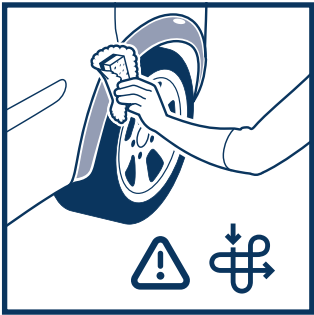
Wipe Q² TRIM EVO onto the surface in a criss-cross pattern. Ensure a thick layer has built up.
