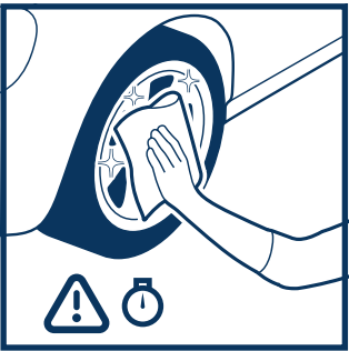
Use Q²M PREP before applying the coating (isopropyl alcohol does not fully degrease the surface).
